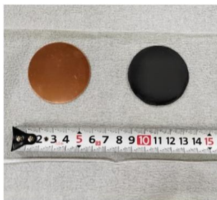
Figure 4. Photo of black body material adopted for the heat transfer analysis and Cu solid disc before splaying black body spray [14,15].
