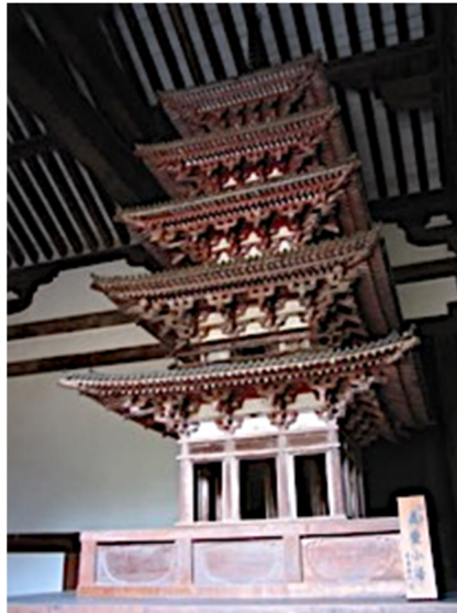
Figure 26. The remaining original 1/5 scale design model of Kairyuouji Pagoda, Japan.
