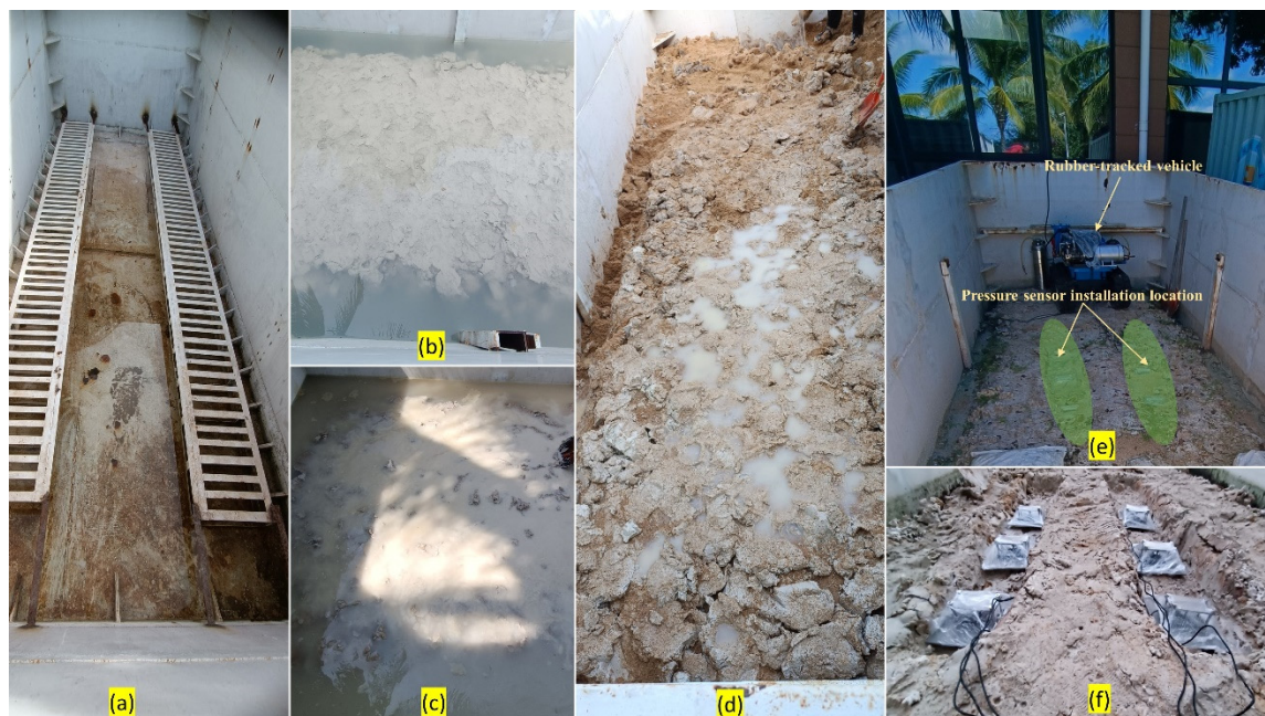
Figure 3. Experimental setup for Soil Bin and pressure sensor installation location (a) Soil Bin used for the experiment, (b) Diatom soil in soil bin, (c) Bentonite soil in soil bin, (d) Sand gravel mixture mixed with bentonite soil, (e) Tracked vehicle and pressure sensor installation location, (f) front, mid, and Rear pressure sensor location in soil bin.
