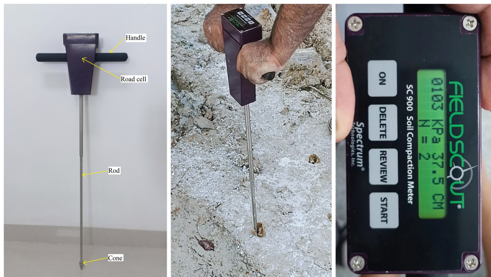
Figure 4. Cone penetrometer and sampling by cone penetrometer.
