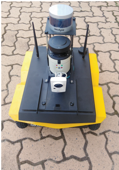
Figure 1. Jackal with RGB Camera [Autonomous Lab @ UNSW Canberra].
