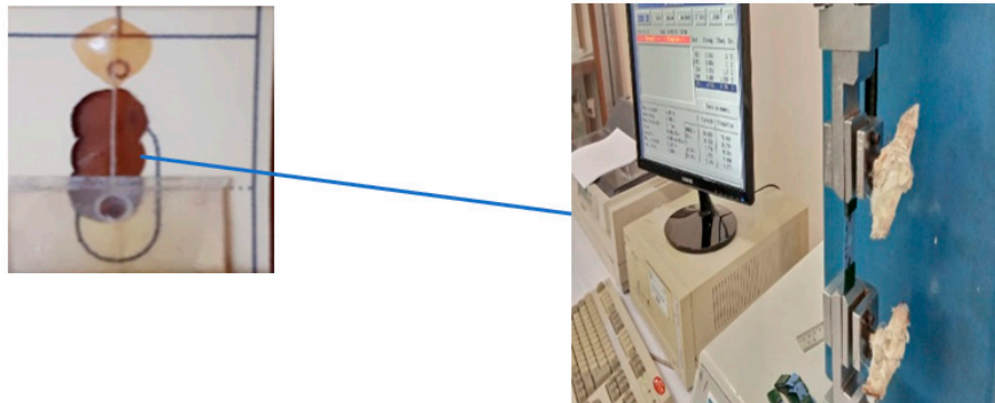
Figure 4. IFSS and Tensile Strength Single Fiber Test.
