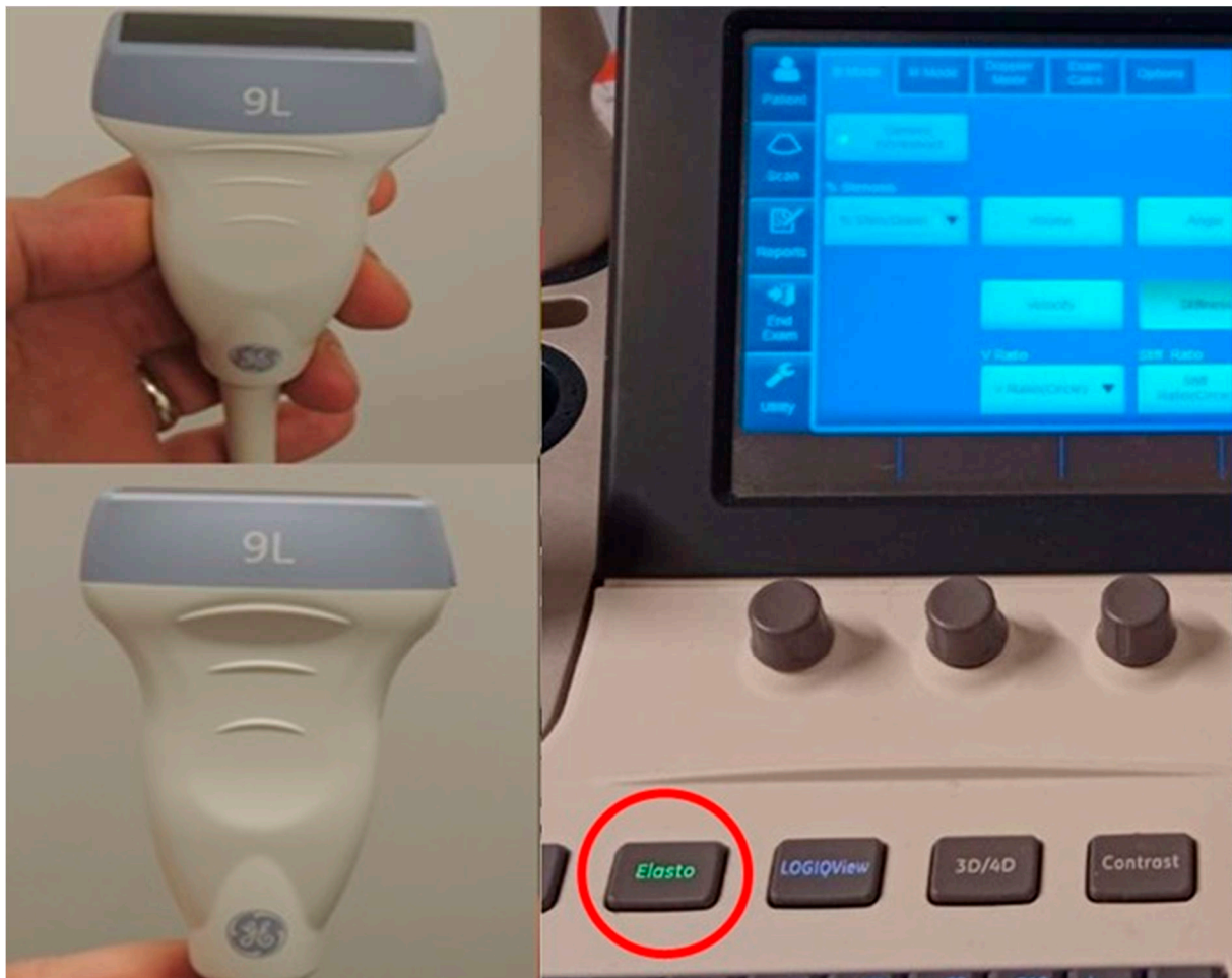
Figure 1. Touch panel and button panel of GE Logic S8 brand/model USG device with elastography software (elastography button is circled in red on the right) and a 9 Mhz linear probe with hardware elastography features (shown from two different directions on the left).
