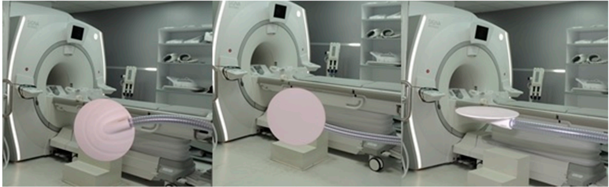
Figure 3. The apparatus called "passive driver," which is one of the extra equipment for MR-E examination, is shown from the back(left), front(centrum), and side(right) in three images from left to right.
