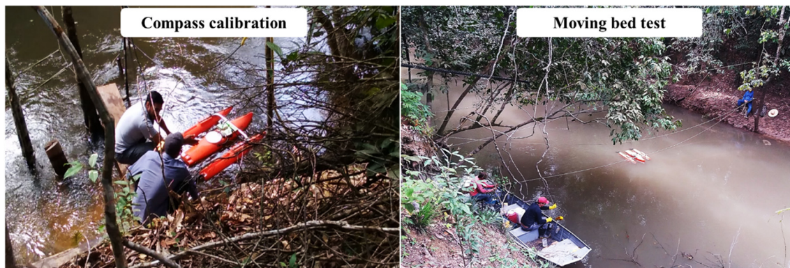
Figure 4. Compass calibration and stationary moving bed test with ADCP RiverRay .
