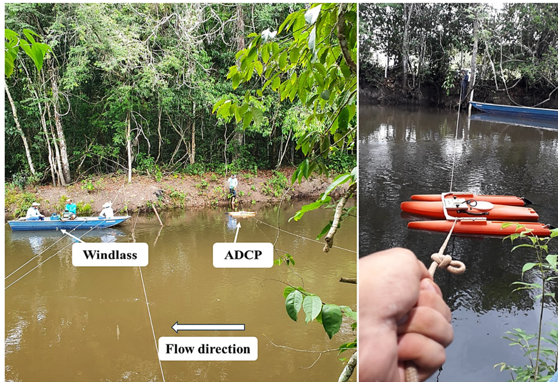
Figure 5. Flow measurement with hydrometric windlass and ADCP in parallel hydrological cross-sections.
