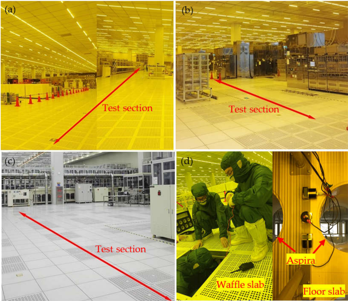
Figure 3. Placement of test points on the second floor: (a) Test section 1 #; (b) Test section 2 #; (c) Test section 3 #; and (d) Installation of sensors on the second-floor slab.
