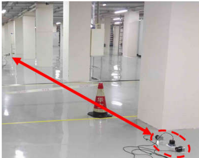
Figure 2. Installation of sensors on the first-floor slab.
