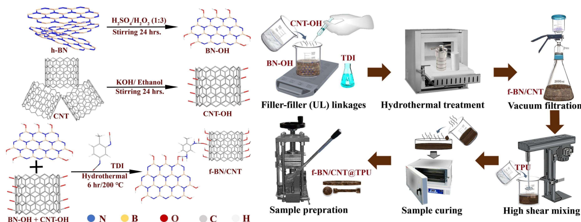
Figure 20. (a) Diagrammatic scheme of the exfoliation and hydroxylation of h-BN and CNT distributions respectively. (b) Labeled Diagrammatic representation for the fabrication of f-BN/CNT@TPU framework. (reprinted with permission from reference [113] Copyright 2023, Elsevier).
