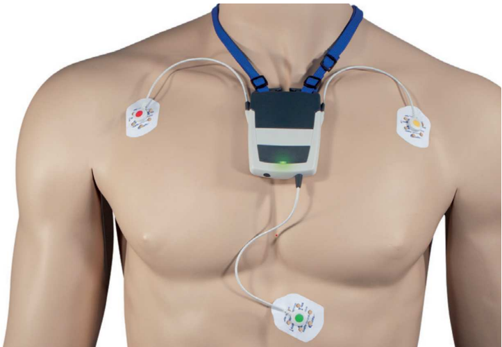
Figure 5. Custo med flash 500/510 3-Channel Holter used for data acquisition of our custom dataset.
