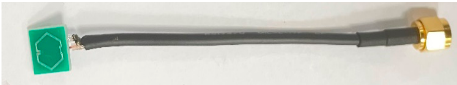
Figure 8. Antenna prototype fed by a 50-Ω RF mini coaxial cable.
