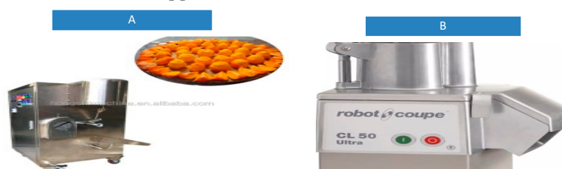
Figure 3. Equipment for processing persimmon fruits before drying them: A- a machine for peeling; B- a machine for cutting into slices of various thicknesses.
