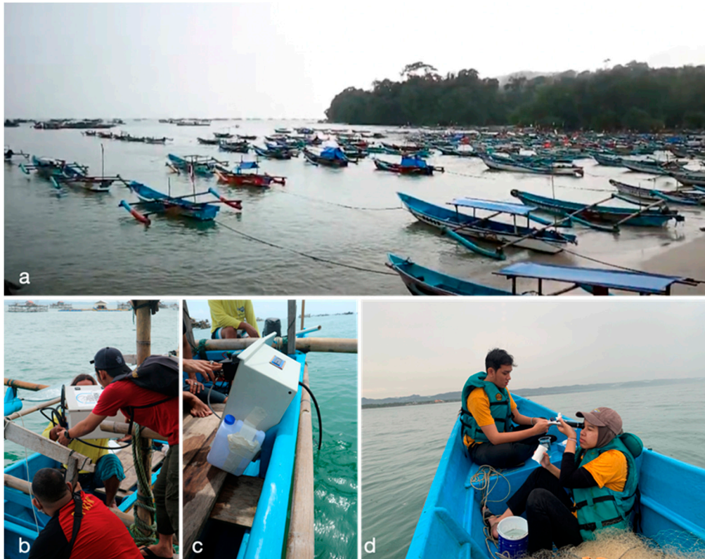
Figure 5. Sea trial in Pangandaraan beach, a) sea condition during the test and type of wooden boat used, b) team and NOBEL-BOX mobilization, c) seawater pumped into the instrument (black water hose), d) measurement with other portable instruments in the front of the ship.
