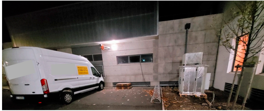
Figure 7. External view of the Raman lidar system MARCO (on the right portion of the figure) during its deployment in Port-Saint-Louis, together with the van used for its transportation (on the left portion of the figure).
