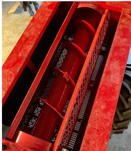
Figure 2. Particular of the threshing system adopted in separation machine.
