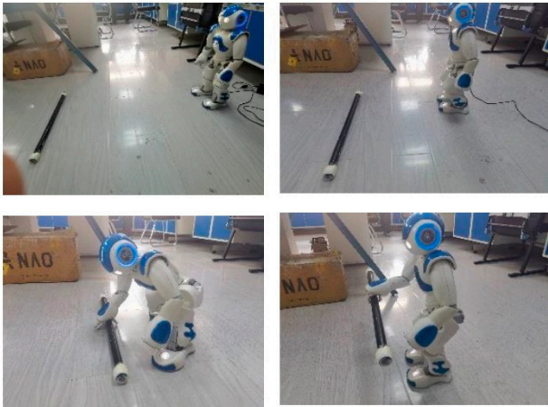
Figure 13. NAO robot grasping process.
