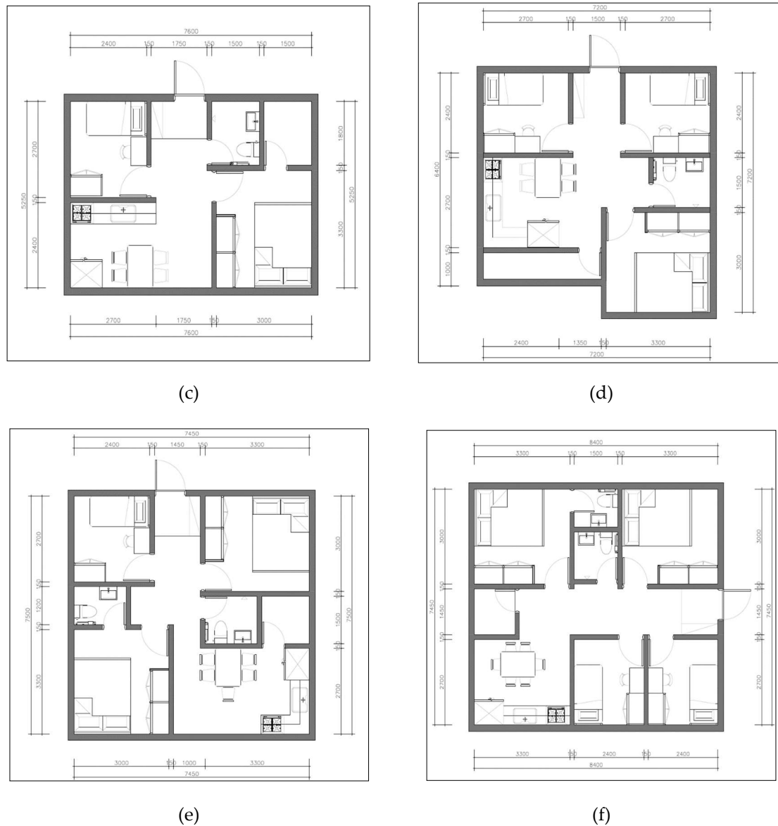
Figure 2. Design simulation of minimum housing standard per household composition (unit: mm): (a) 1-person(18m 2 ); (b) 2-person(30m 2 ); (c) 3-person(40m 2 ); (d) 4-person(48m 2 ); (e) 5-person(56m 2 ); (f) 6-person(63m 2 );.
