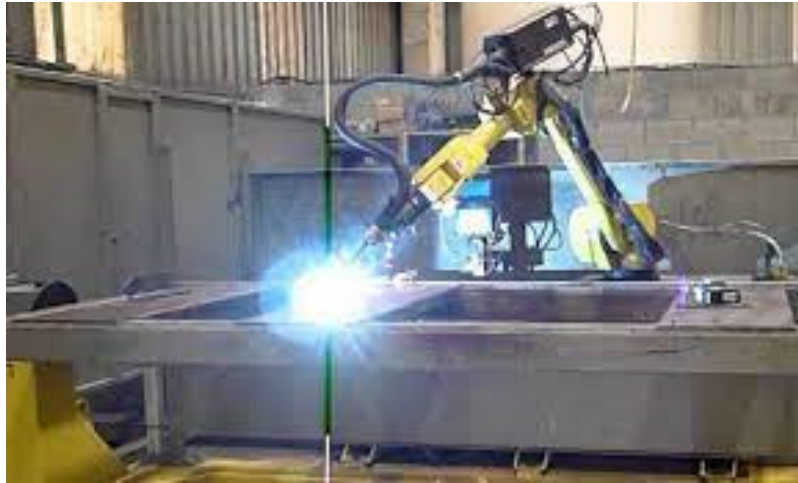
Figure 2. Welding tool mounted on the end member of the robotic system.
