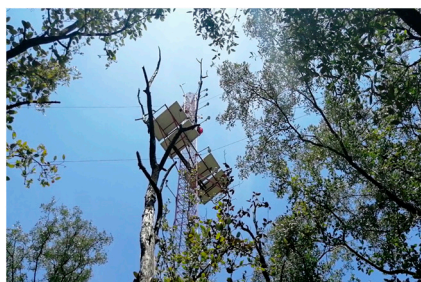
Figure 2. Micrometeorological tower in the Juan Díaz mangrove ecosystem as seen from below.
