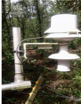
Figure 4. Temperature and relative humidity probe encased in radiation shield.
