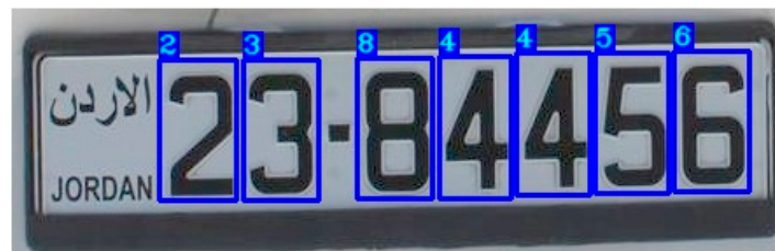
(a) Outputs of the Re-trained YOLOv3 Model for the Jordanian LPR (CR) Task.
