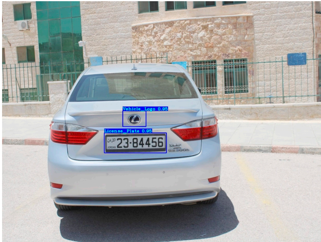
Figure 2. Outputs of the Re-trained YOLOv3 Model for the Jordanian LPD and VLD Tasks.
