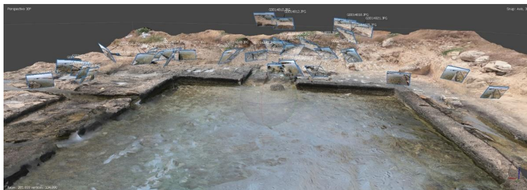
Figure 8. Southern sector of the Lambousa ft reconstructed with the photogrammetric method. The width of the fishtank is 13.6 m, while the length is 23.8 m (see also Fig. 7).
