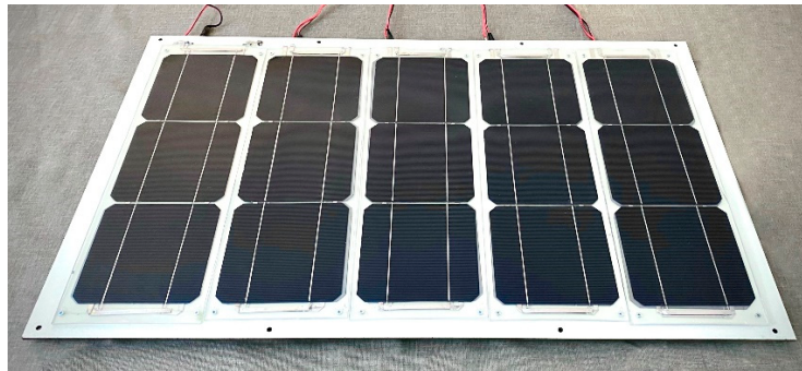
Figure 5. A picture of the home-made illuminance sensor (PV-surface), utilized for estimating the level of the sunlight passing through the PV-skylight (on the underlying surface area), in five different zones.
