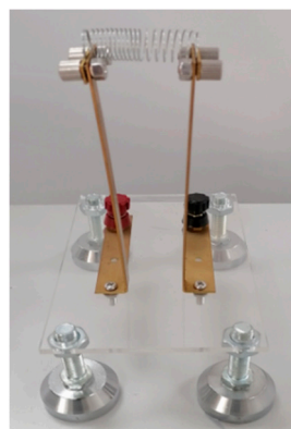
Figure 4. Structure and fixing method of hot wire.
