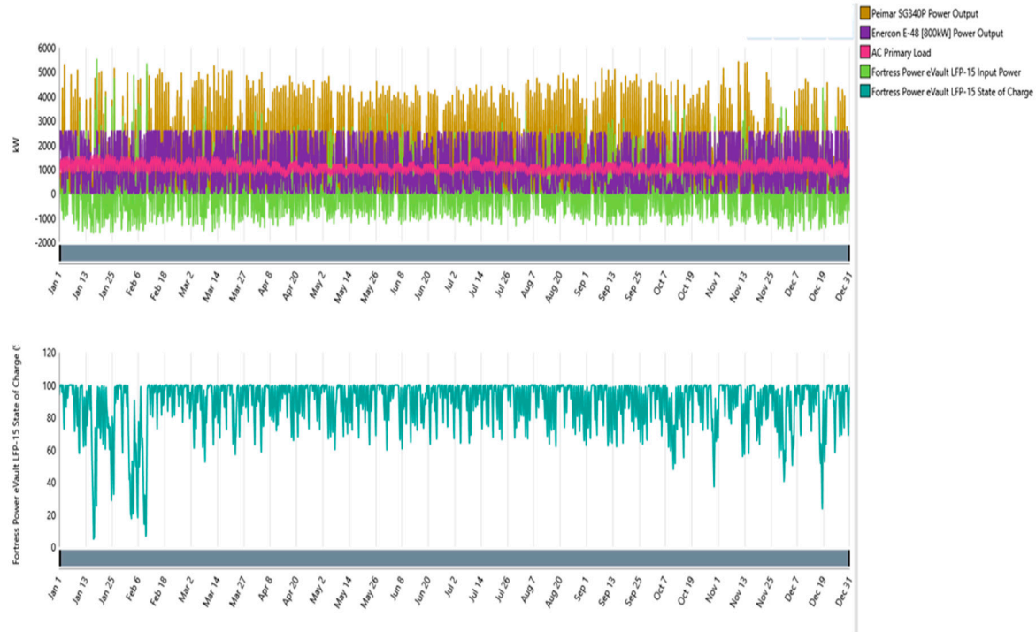
Figure 16. Scenario 1 Solar PV, Wind turbine and Battery power output along with the power demand and Battery state of charge.
