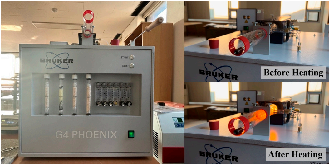
Figure 4. Hydrogen charge measurement test using gas chromatography.
