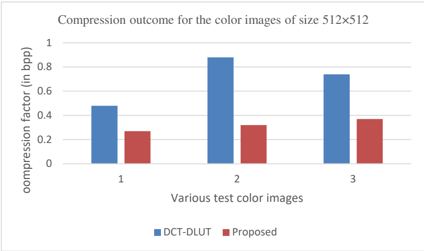
Figure 20. Comparison of various compression techniques used on the different color test images: 1- airplane, 2-pepper, and 3-Lena.
