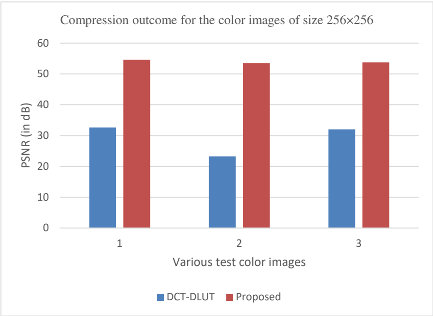
Figure 21. Comparison of various compression techniques used on the different color test images: 1- Couple, 2-House, and 3-Zelda.
