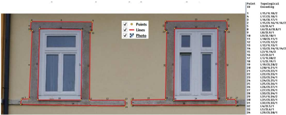
Figure 7. a) Digital sketch of building on Figure 6 (zoom) – left b) Points list with topological codes – right.
