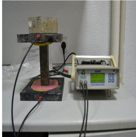
Figure 3. Electrical resistivity test.
