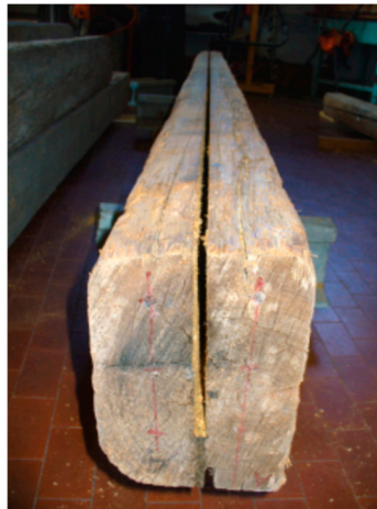
Figure 2. Beam n. 3 after the third groove to 75% of the depth.
