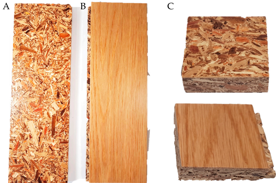
Figure 4. Forest biomass-based composite applied in a Panel (A) and Floor (B), as well as test pieces of each prototype (C).
