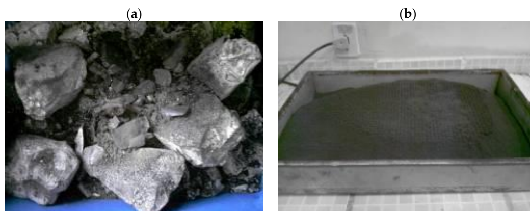
Figure 2. Remaining mixture ( \text{Na}_2\text{CO}_3 + coke): (a) before comminution; (b) after comminution.
