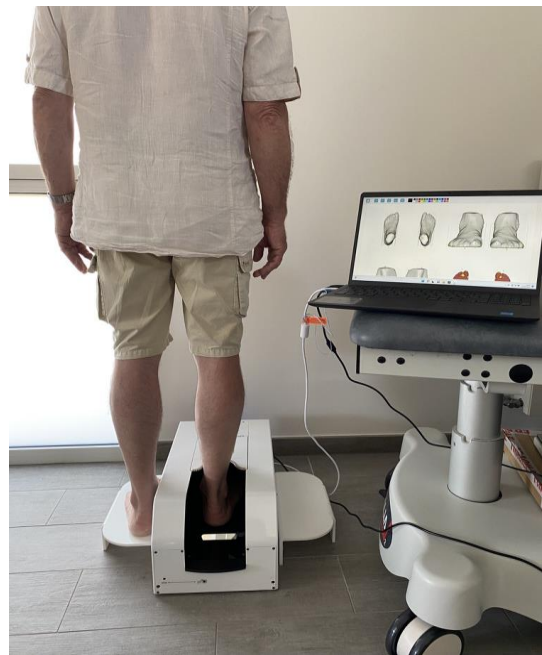
Figure 2S. Subjects were positioned standing on both feet (one foot in the scanner, and the other foot on a footrest at the same height).
