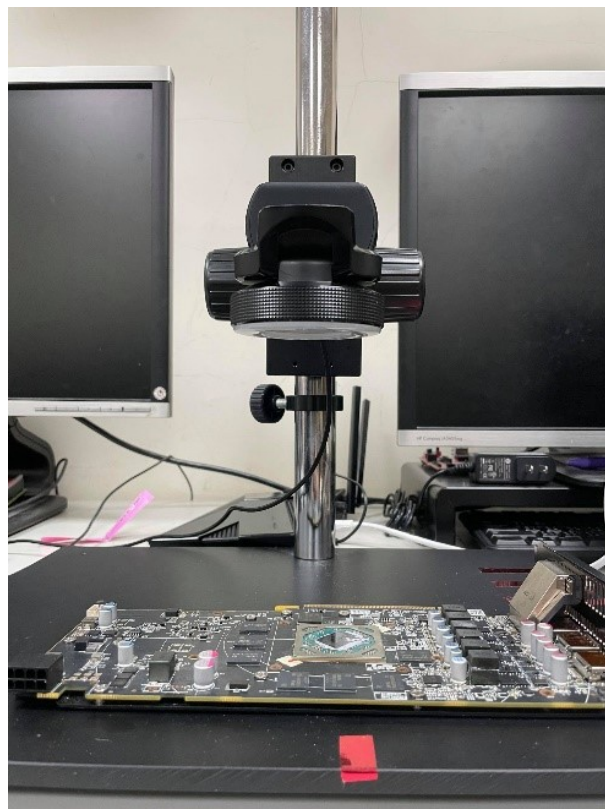
Figure 6. The setup of the experiment. A high resolution industrial camera is adopted for the acquisition of images from the PCBs.
