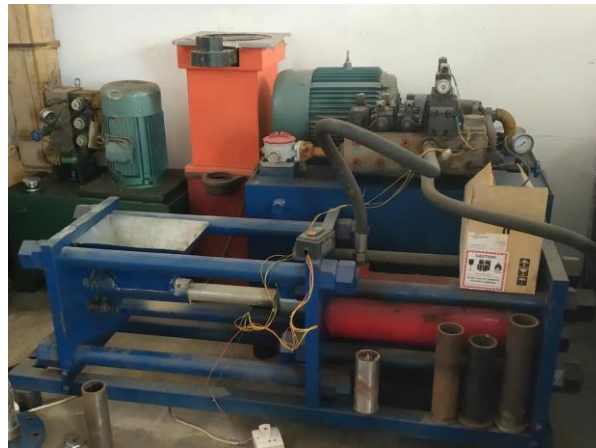
Figure 1. The structure of hydraulic briquetting machine with plunger.
