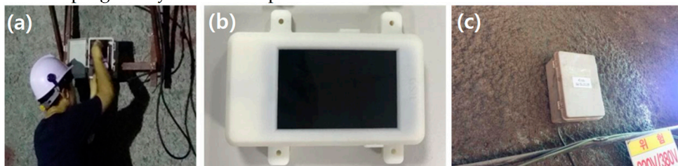
Figure 5. Bluetooth scanner (Gsil-S0011) for communication based on wearable devices (Gsil-B0011): (a) Installation; (b) Inner module; (c) Installed device with casing.
