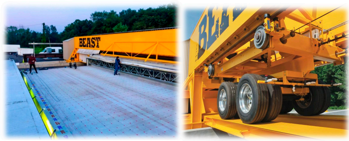
Figure 18. The bridge deck in the BEAST facility (left) and the dual-axle carriage (right).
