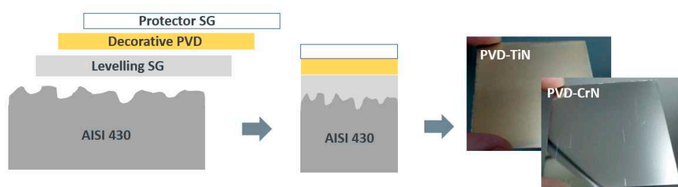
Figure 9. Schematic drawing of the multilayer system and pictures of the gold and silver finish reached under the top coat.
