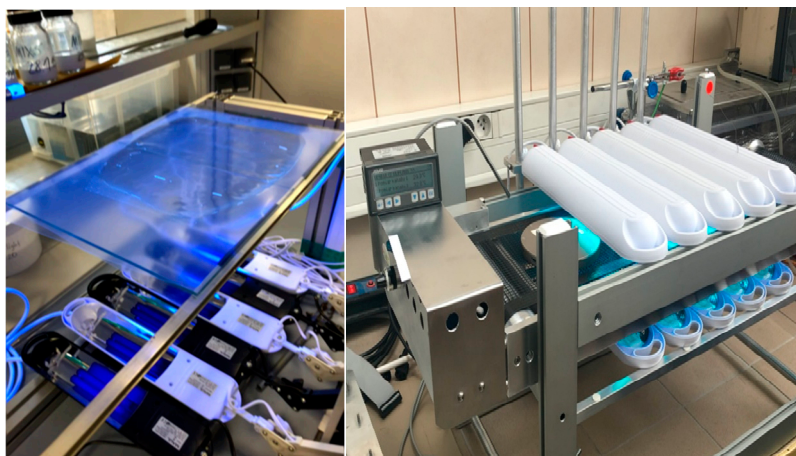
Figure 3. UV-initiated crosslinking of photoreactive transfer tape.
