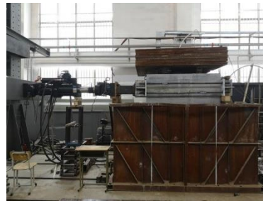
Figure 1. Schematic diagram of lateral cyclic loading rig used for model test and the specimen instrumentation (unit: mm): (a) RC pile group specimen; (b) single pile specimen; (c) Schematic views of RC pile group test system.
