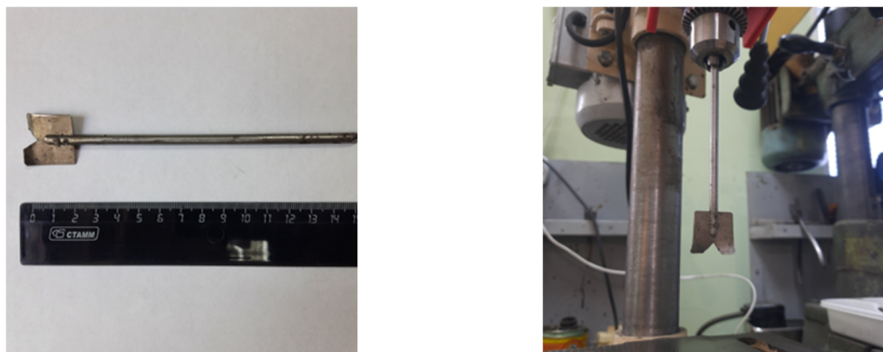
Figure 1. The blade on the pin (left) inserted into the drill chuck (right).
