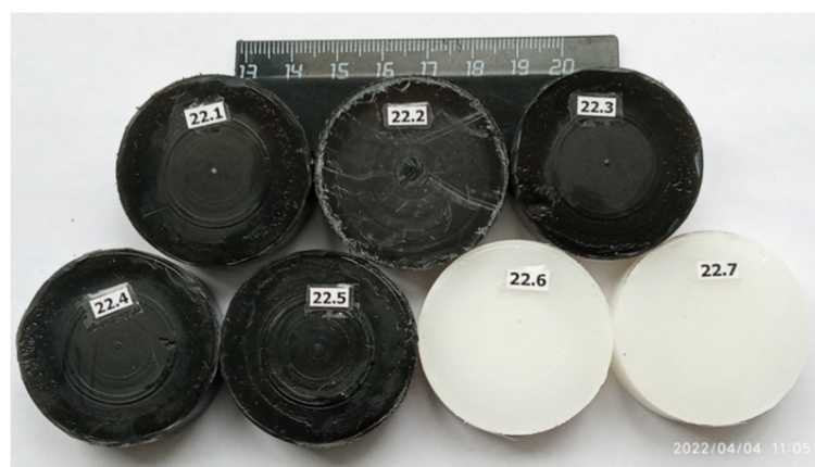
Figure 2. Disk-shaped compacts manufactured by the SIS method: white samples from pure UHMWPE, black samples from UHMWPE with carbon nanoadditives.
