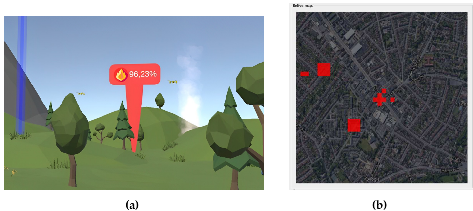
Figure 28. Left: The VR-HSI interprets the values from the trust map and places a beacon next to a disaster. Right: The Desktop-HSI marks significant values on the trust map with a red square.
