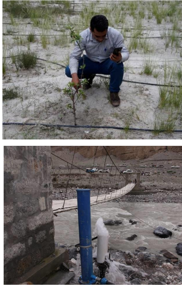
Figure 7. Measuring emitter discharge (left image) and Hydraulic Ram Pump under operation (right image).
