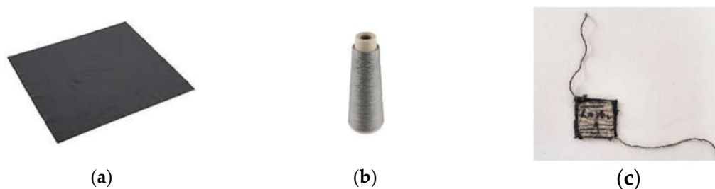
Figure 3. Materials used for sensor development: (a) conductive stretchable fabric, (b) silverplated conductive thread, (c) designed sensor.
