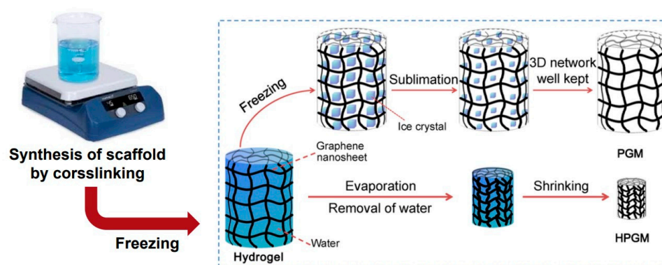
Figure 1. Fabrication of CMC porous scaffolds containing silk fibroin. Schematic diagram of the fabrication process of fibroin/CMC hybrid scaffolds obtained by freeze-drying method.
