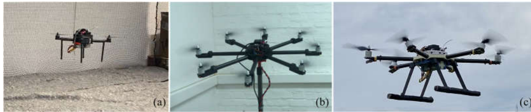
Figure 6. Motor mixer verification experiment: (a) Quadrotor; (b) Ocotorotor; (c) Fully actuated hexarotor.
