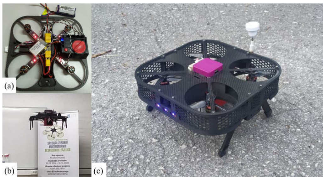
Figure 9. Phases of assembling the quadrotor UAV: (a) Testing the propulsion elements using a servo tester; (b) Preliminary testing of the supporting airframe; (c) Ready-to-fly experimental platform.
