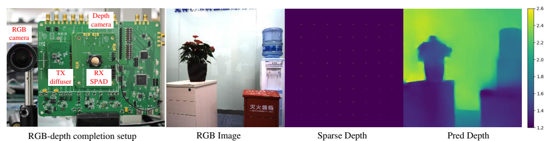
Figure 11. The result of our hardware system. From left-to-right: RGB-depth completion setup, Guidance RGB image, the sparse depth map and the predicted depth map from our network.
