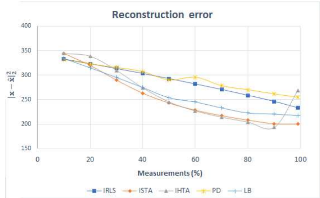
Figure 11. Error in the reconstruction of Fig. (3) as a function of the number of measurements for each algorithm.
