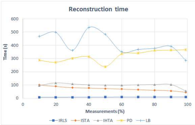
Figure 10. Reconstruction time of Fig. (3) as a function of the number of measurements for each algorithm.
