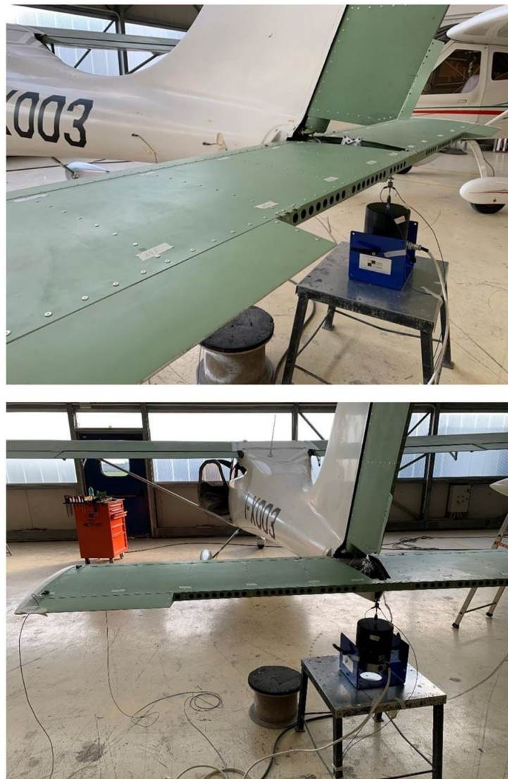
Figure 12. Test setup Vibration Tests Horizontal tail twin-seat ultralight aircraft.
