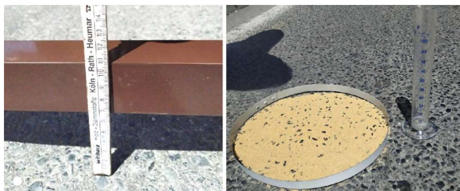
Figure 1. Visualizing data collection with sand patch and lath/nail method.
