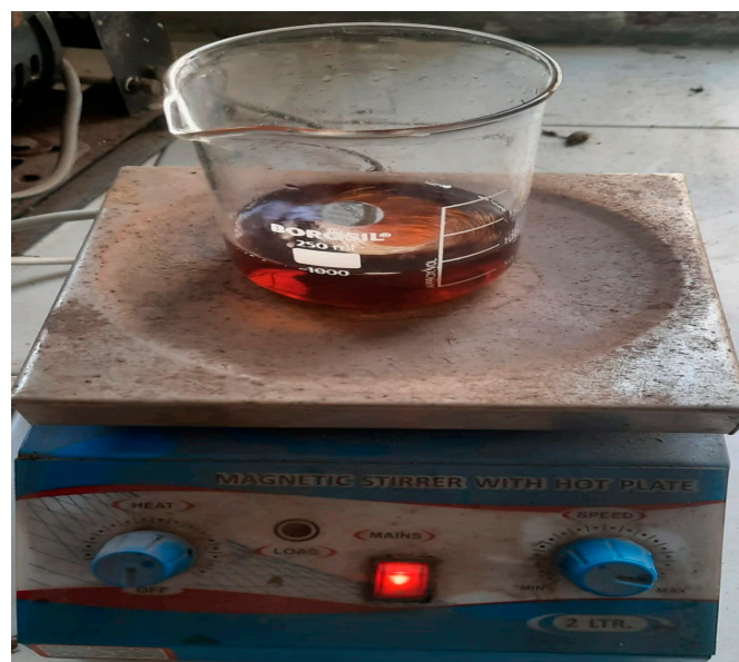
Figure 3. Magnetic stirrer while preparing \text{TiO}_2 NPs.
